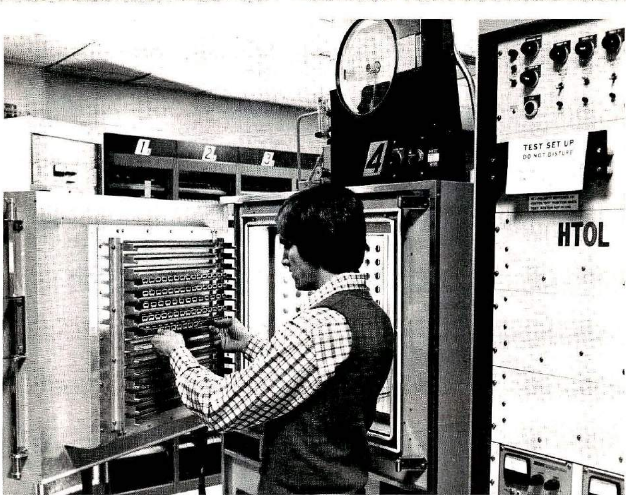
Complex integrated circuits such as microprocessors and memory devices must have high reliability. Most manufacturers "burn in" complex devices by operating them at high temperatures with power on for up to 180 hours. Those ICs that are likely to fail do so in the stress of temperature plus power. Integrated circuits that pass the burn-in period can be expected to have a long, trouble-free lifetime.
