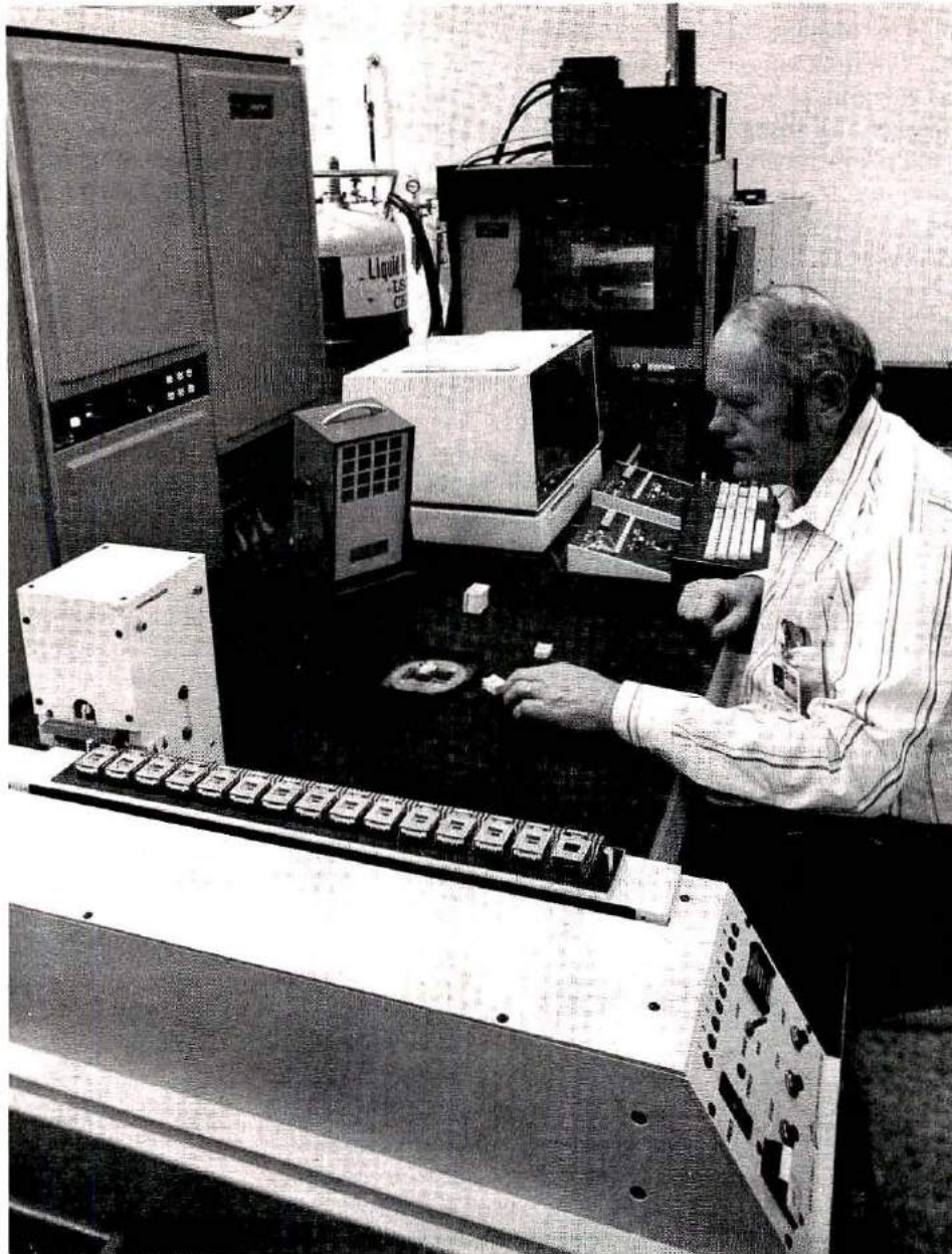
Digital integrated circuits require complex test equipment. Shown here is a Fairchild Sentry 7 in use at Raytheon Corp. The large desk contains digital driver/detectors for each pin of the IC package. A tester such as this costs $500,000.
