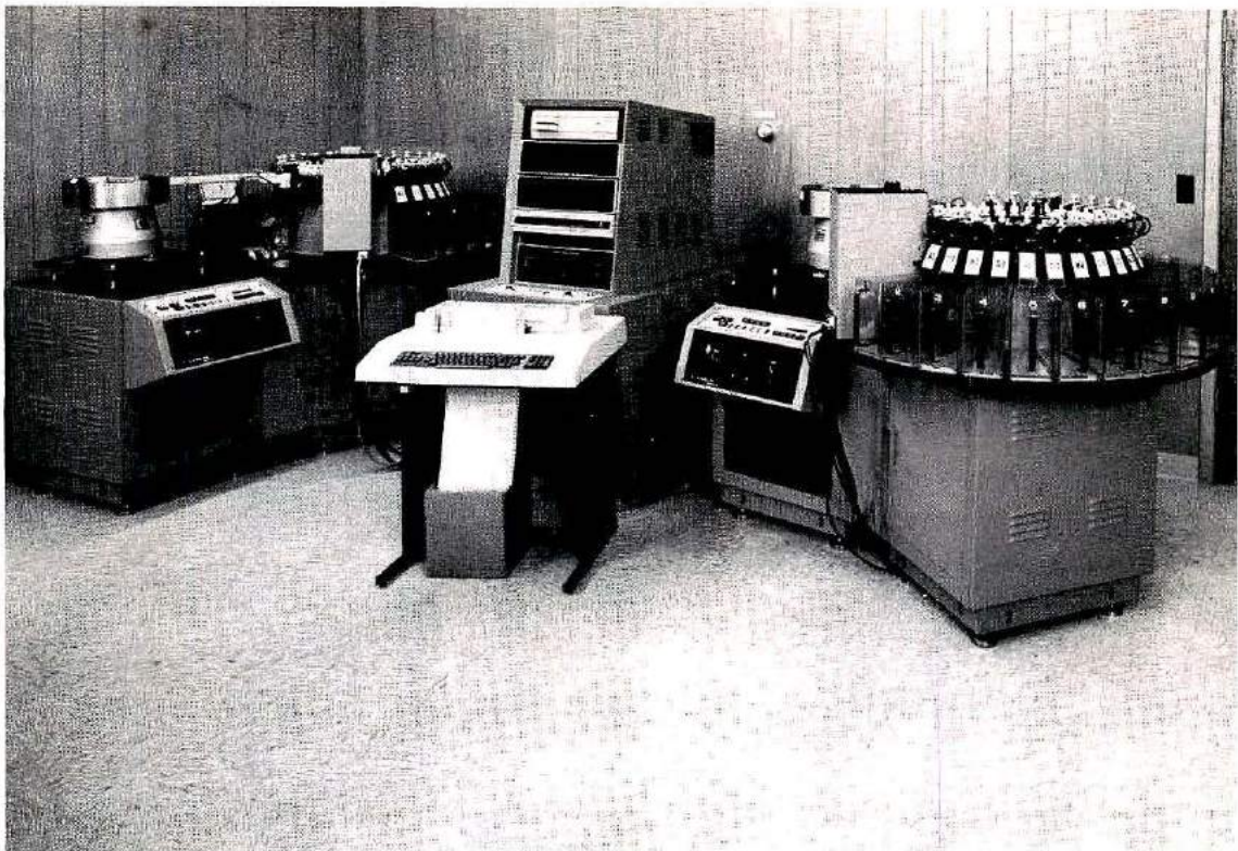
Another way that semiconductor manufacturers bring down costs is by using automatic test and handling equipment. Shown here is a test system built by Lorlin Industries of Danbury, Connecticut, for Texas Instruments, Singapore. The unit tests and sorts dual-gate MOSFETs at the rate of 10,000 per hour.
